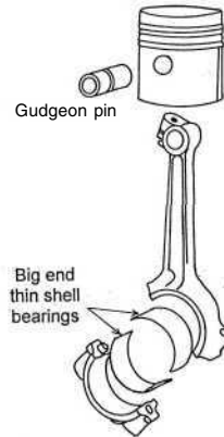
Fig 5.13 Split shell bearings and a gudgeon pin
